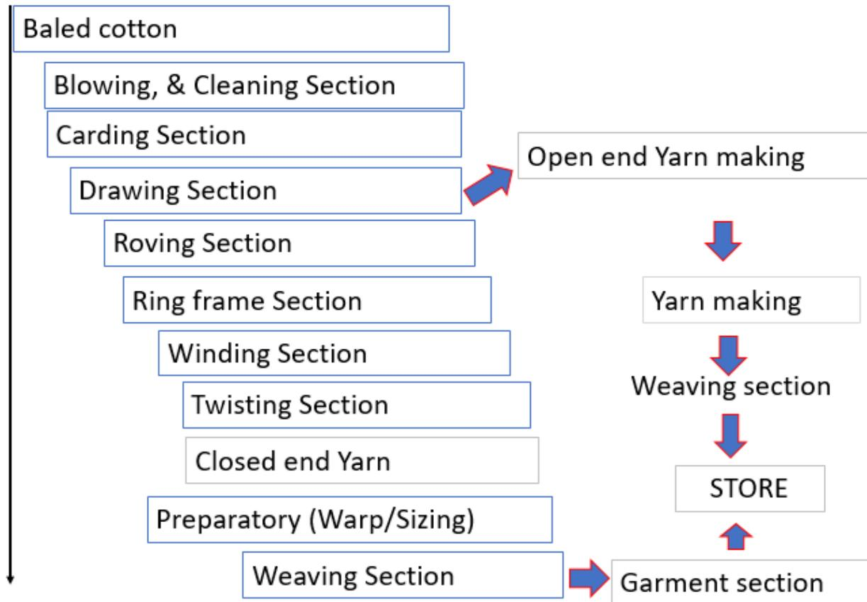
Figure 1: The textile mill flow process (the process involves two technologies: closed ended, the very traditional one involving different processes in different machines; the open ended that integrated the tasks of roving, ring frame winding, and twisting in one row of machines. The output in both cases is yarn production)
