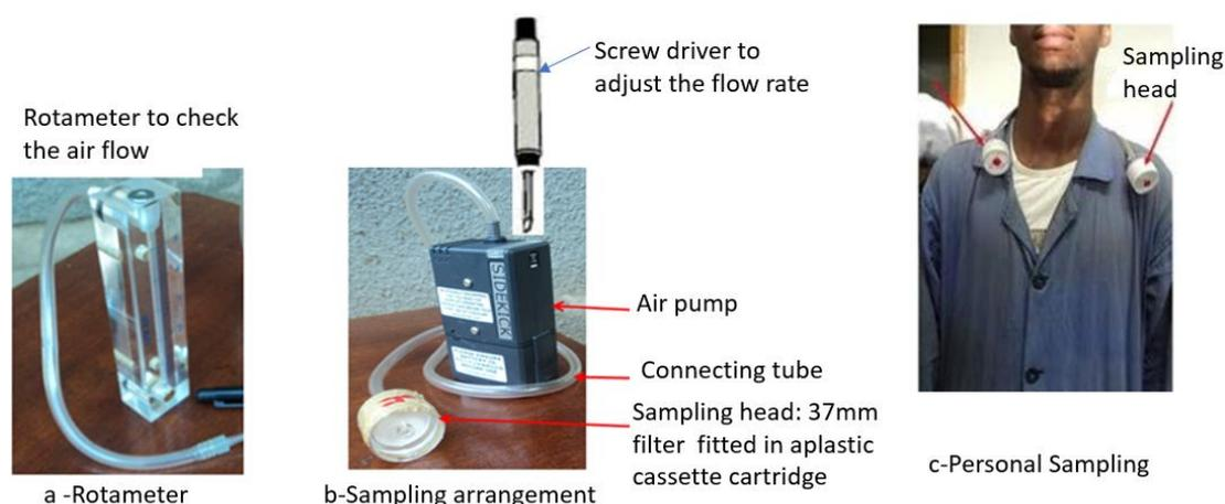
Figure 2: Cotton dust sampling arrangement
